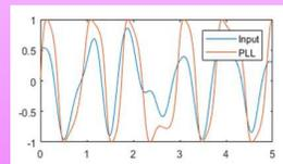
Figure 2: EEG signal (input) vs PLL output
